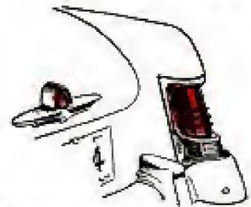
MERCURY extended its rear fenders over the top of the taillight unit
